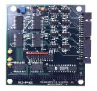
D/A Converters and buffer amplifiers - The card employs up to four Analog Devices AD7228A eight-channel D/A converters. Output resolution is 8-bits with  $\pm 1$  LSB nonlinearity and relative accuracy. The voltage output settling time of 5 μs and a slew rate of 2 V/μs.
